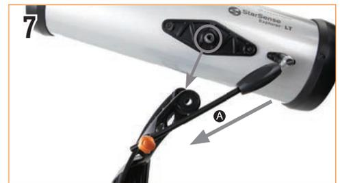
7 Slide the altitude rod **A** into the rod guide on the mount and lower the altitude hubs on the telescope tube into the cradles on the top of each yoke arm.
