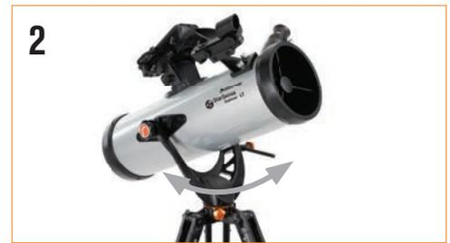
Hold the tripod leg with one hand and grab the telescope tube focuser and move it left or right as desired. The amount of tension you feel when moving the telescope can be adjusted by tightening or loosening the knob to a level that is comfortable for you.
