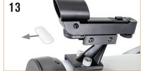
**13** There is a small clear plastic tab inserted between the battery and the contact. This was included to prevent the battery from discharging during shipment. Pull this out to allow your battery to work.
