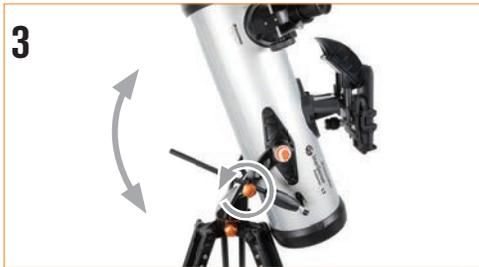
To move the telescope up and down, hold the focuser of the telescope in one hand and loosen the knob on the slow motion rod guide. The telescope can now be moved up or down as desired. When you are close to your target, tighten the knob to secure the telescope in place.
